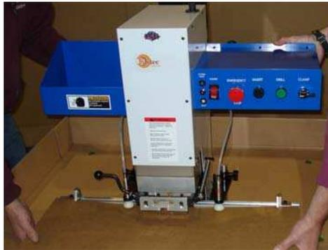
4.) Hook up the vacuum/dust collector. Use the 4" tube for a shop system or the 2" tube for a portable shop-vac.
