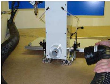
6.) **STAY CLEAR OF THE FRONT OF THE MACHINE.** Plug the air hose into the shop air supply. **CAUTION:** The boring head will quickly move to the up position and the work-piece hold down clamps may actuate to the down position.
