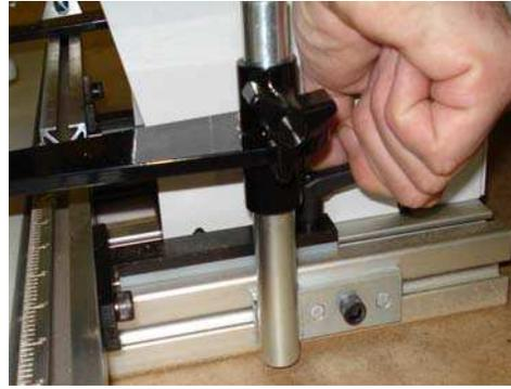
13.) Adjust the pneumatic hold down clamps. Loosen the knob to move the bracket up and down or to swivel to the left or right. Loosen the socket head cap screw holding the shaft assembly to the extruded aluminum machine leg to move front to back. To move the hold down clamp further away from the center of the machine take the assembly off of the extruded aluminum leg and affix into the slot on the back rail.
