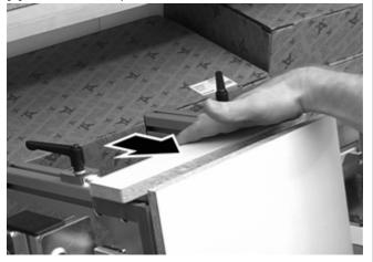
[3] Clamp the rear panel with depth gauges. Tighten the lever.
