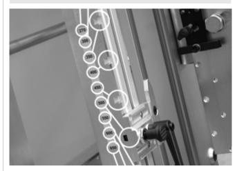
[2] Snap bracket into the desired notch. Secure the position by tightening the lever.
