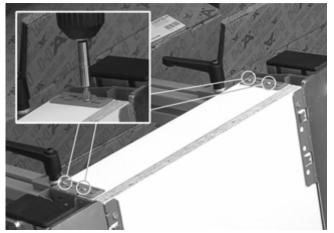
[3] Open both clamping levers. Remove the drawer.
