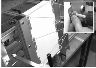
[2] Fix screws 3.5 x 15 mm (#6 x 5/8"-Flathead) into rear panel (quantity as required).
