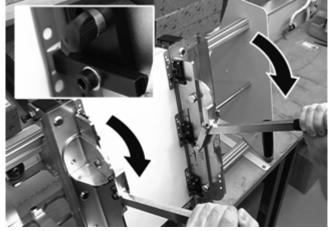
[3] Fix screws 3.5 x 15 mm (#6 x 5/8"-Flathead) into rear panel (quantity as required).
