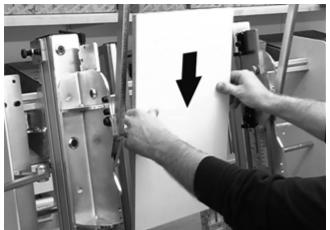
[2] Push the back panel flush to the bottom.
