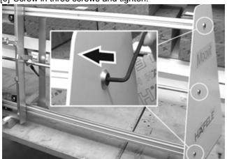
[3] Attach both clamping arms with two included screws (length of 30 mm). Observe the position (see image).
