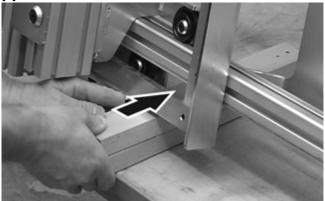
[2] Unscrew three screws. Remove the right metal plate.
